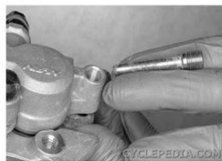
Remove the pad pin with a 5 mm Allen.
